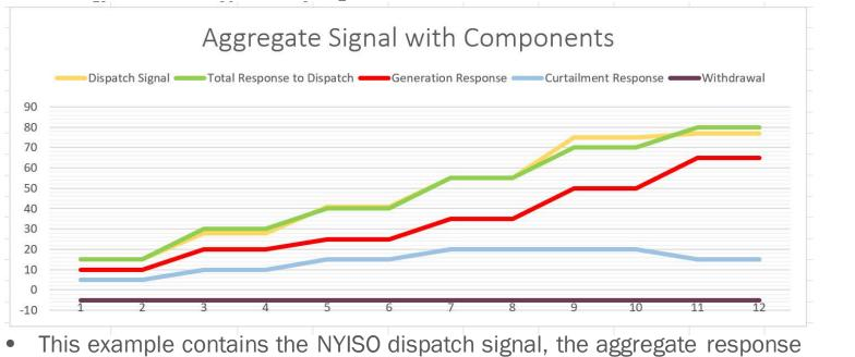
This example contains the NYISO dispatch signal, the aggregate response signal and the sub-component signals for settlements
